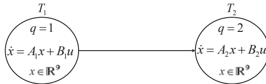
Figure 6.8.: Hybrid automaton: communication \rightarrow no communication.
