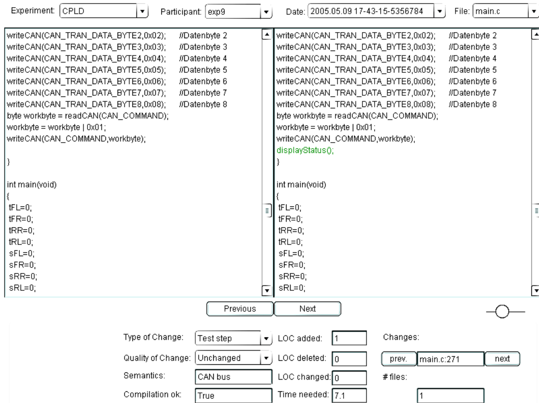
Figure 15.3: Graphical user interface of the source stepper applications
