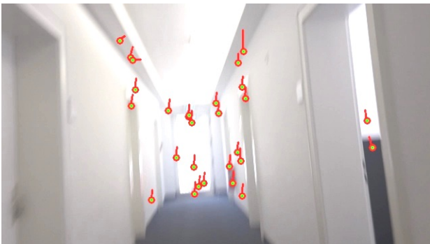
Fig. 1: Vector movement of equal feature points between two successive frames.
