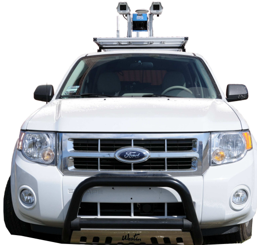
(a) Ford Escape Hybrid – ByWire XGV’s sensors: On the roof there is a stereo vision system alongside with a single layer laser scanner mounted for perceiving the vehicle’s surroundings in front of the car.
