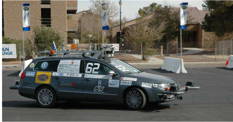
Figure 2.1: Autonomously driving vehicle “Caroline” at the 2007 DARPA Urban Challenge in Victorville, CA. This vehicle was the contribution from Technische Universität Braunschweig for that international competition. The vehicle was a 2006 Volkswagen Passat station wagon which was modified for driving autonomously in urban environments. Detailed information about the vehicle, its modifications, and its performance during the competition can be found at [122].
