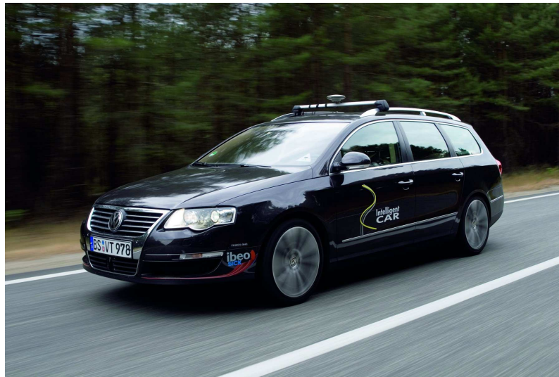
Figure 2.2: Vehicle “Intelligent Car” from Volkswagen at the company’s own proving ground in Ehra. This vehicle was able to drive automatically on highways by continuously evaluating its surroundings to derive suitable driving propositions for safely passing slower moving vehicles for example. Further information about the vehicle can be found at [7]; image credit: Volkswagen Corporation.
