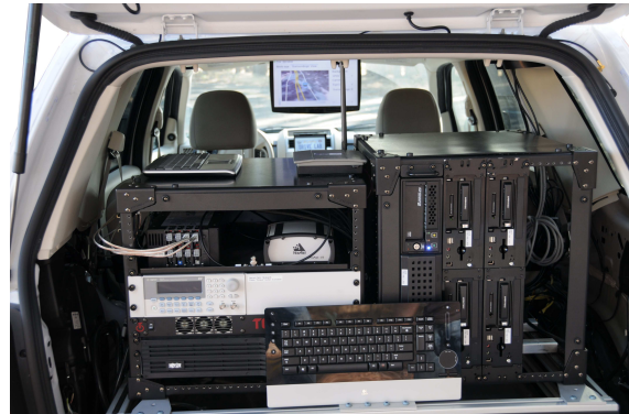
(b) Ford Escape Hybrid – ByWire XGV’s trunk: The incoming data is processed on several computers which are mounted in the rack on the right hand side of the trunk. On the left hand side, an IMU for providing highly precise position data is mounted as well as a waveform generator to provide a synchronization signal to trigger the independent cameras of the stereo vision system.
