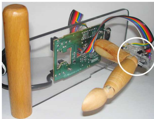
Fig. 1. Prototype constructed from parts of a manikin with an optical mouse sensor, used in order to measure joint rotation
