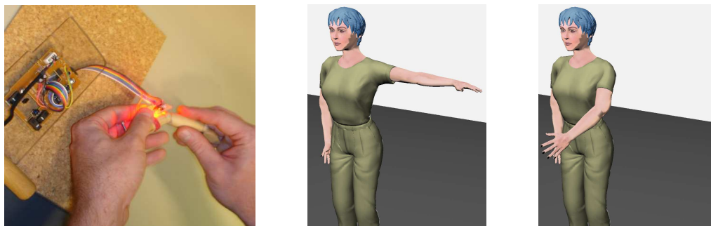
Fig. 5. Example of using O.M.I. (left) to bend the arm of a virtual character (middle and right)
